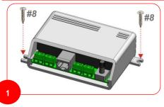
Secure the LMPS-Dimmer with #8 screws.
